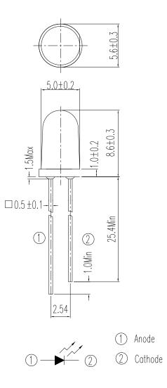
Note: Tolerances unless dimensions ±0.25mm
