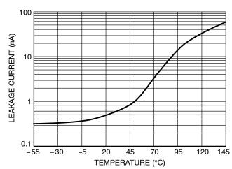
Figure 3. SD05 Typical Leakage Current versus Temperature
