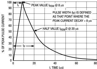
Figure 5. Pulse Derating Curve
