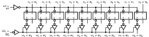
Please note that this diagram is provided only for the understanding of logic operations and should not be used to estimate propagation delays.
