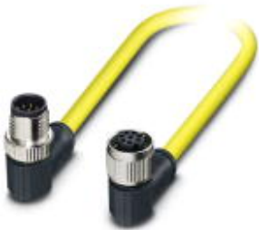
Sensor/Actuator cable, 8-position, PVC, yellow, Plug angled M12 SPEEDCON, A-coded, on Socket angled M12 SPEEDCON, A-coded, Cable length: 1.5 m
