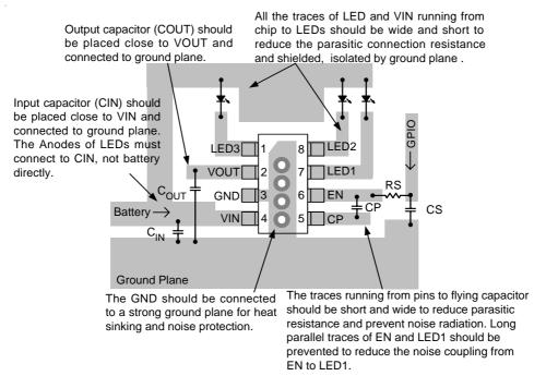
Figure 4. PCB Layout Guide.
