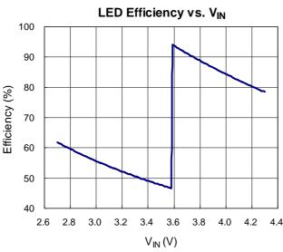
Figure 3. Efficiency of RT9363. (I<sub>LED</sub> = 60mA, V<sub>F</sub> = 3.45V)
