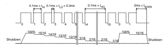
Figure 1. Brightness control by pulse dimming. RT9363 implements 16 steps brightness control
