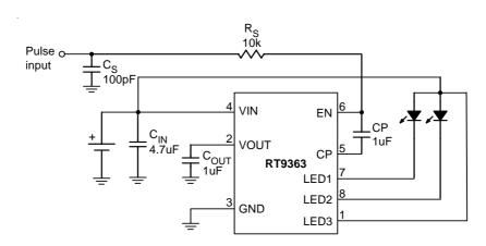
Figure 2. For 2-WLEDs Application Circuit
