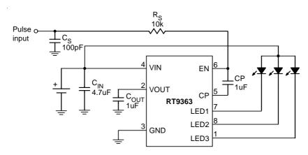
Figure 1. For 3-WLEDs Application Circuit
