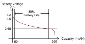
Figure 2. Li-ion Battery Energy Capacity Versus Battery Voltage.
