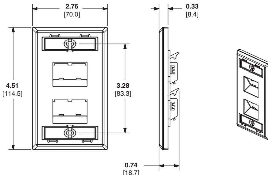
Dimensions are in inches. [Dimensions in brackets are metric.]
