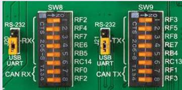
In order to enable USB-UART communication, you must set **J20** and **J21** jumpers in the **USB-UART** position, and enable desired **RX** and **TX** lines via **SW8** and **SW9** DIP switches. For example, if you want to enable USB-UART connection on UART1 module of the default **dsPIC30F4013** chip, you should enable **SW8.1** (RF2) and **SW9.1** (RF3) lines.
