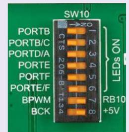
**IMPORTANT:** In order to use PWM back light both **SW10.7** and **SW10.8** switches must be enabled at the same time.
