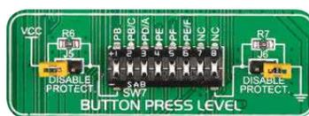
**Figure 10-6:** Button press level DIP switch (tri-state)
