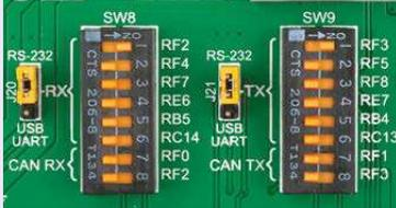
In order to enable RS-232 communication, you must set **J20** and **J21** jumpers in the **RS-232** position, and enable desired **RX** and **TX** lines via **SW8** and **SW9** DIP switches. For example, if you want to enable RS-232 connection on UART1 module of the default **dsPIC30F4013** chip, you should enable **SW8.1** (RF2) and **SW9.1** (RF3) lines.
