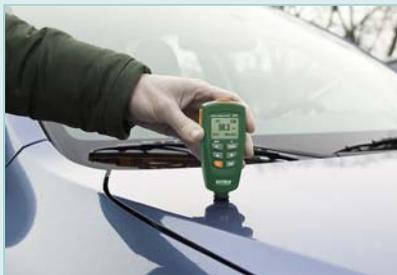
Measuring the thickness of automotive paint
