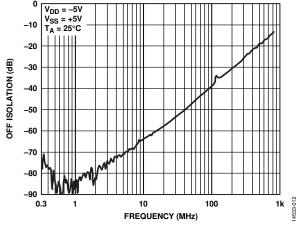
Figure 12. Off Isolation vs. Frequency
