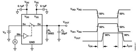
Figure 17. Switching Times
