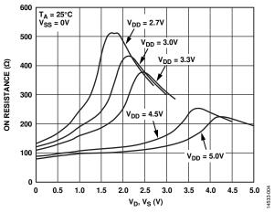
Figure 4. On Resistance vs. V<sub>D</sub>, V<sub>S</sub>; Single Supply
