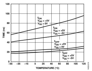
Figure 10.  $t_{ON}/t_{OFF}$  Times vs. Temperature
