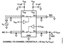
Figure 21. Channel-to-Channel Crosstalk
