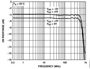
Figure 11. On Response vs. Frequency
