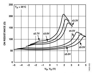
Figure 3. On Resistance vs. V<sub>D</sub>, V<sub>S</sub>; Dual Supplies
