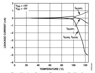
Figure 7. Leakage Current vs. Temperature, Dual Supplies
