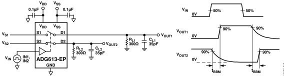
Figure 18. Break-Before-Make Time Delay
