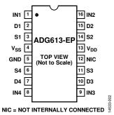
Figure 2. Pin Configuration
