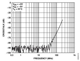
Figure 13. Crosstalk vs. Frequency
