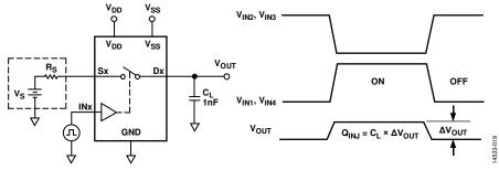
Figure 19. Charge Injection
