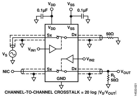
Figure 21. Channel-to-Channel Crosstalk
