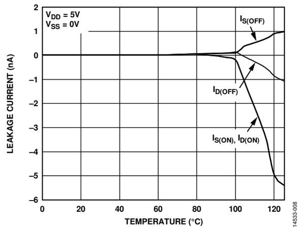
Figure 8. Leakage Current vs. Temperature, Single Supply
