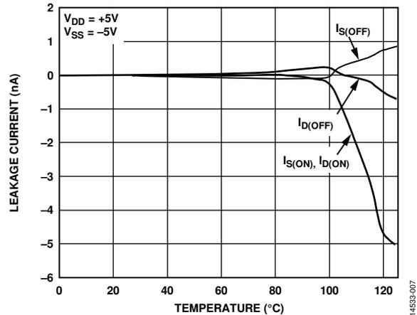
Figure 7. Leakage Current vs. Temperature, Dual Supplies
