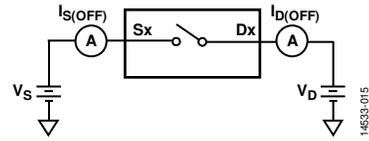
Figure 15. Off Leakage
