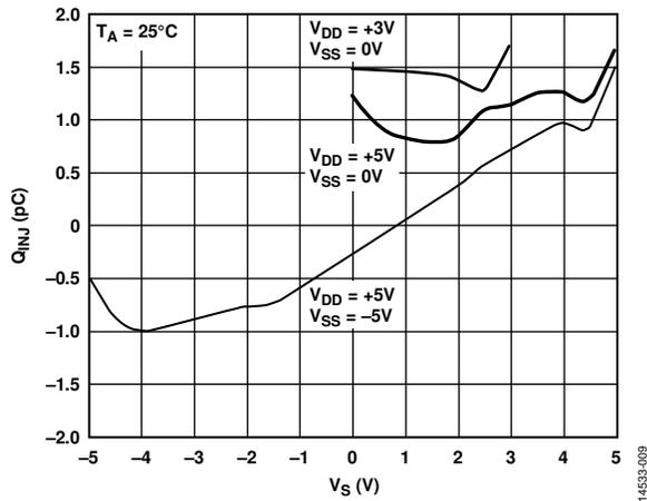
Figure 9. Charge Injection ( $Q_{INJ}$ ) vs. Source Voltage ( $V_S$ )
