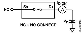
Figure 16. On Leakage
