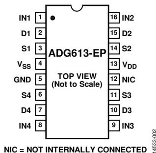
Figure 2. Pin Configuration
