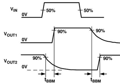
Figure 18. Break-Before-Make Time Delay
