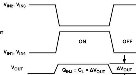
Figure 19. Charge Injection
