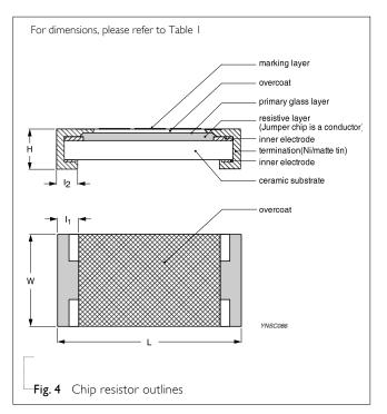
Chip Resistor Surface Mount RC\_P SERIES 0100 to 2512
