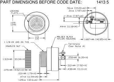
NOTE A: TERMINALS-032 BRASS TIN PLATED, TAPPED FOR #6-32 SCREW. TVD #6-32 NICKEL PLATED BRASS SCREWS INCLUDED. WILL ACCEPT 1/4\* QUICK CONNECT.
