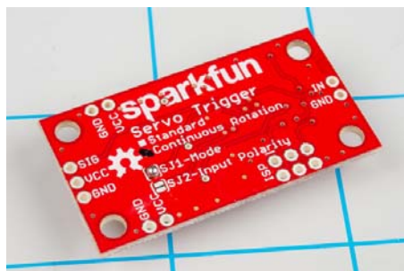
Closing SJ1 to select bistable mode.
