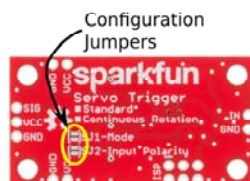
Configuration Jumpers, SJ1 and SJ2.
