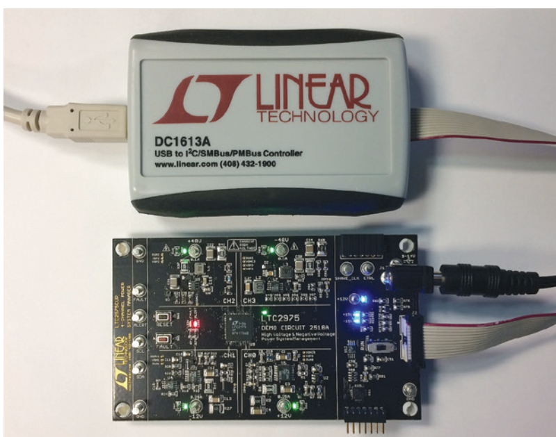
Figure 3. Connecting DC2518A and the DC1613 USB to I 2 C/SMBus/PMBus Controller
