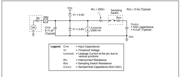
**Note:** CPIN value depends on device package and is not tested. Effect of CPIN negligible if Rs  $\leq$  5 k $\Omega$ .
