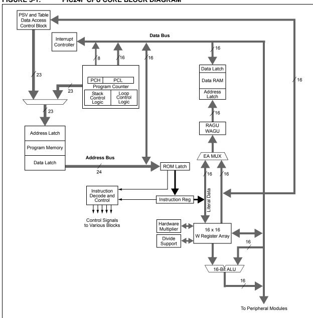
FIGURE 3-1: PIC24F CPU CORE BLOCK DIAGRAM
