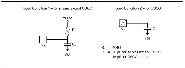
TABLE 26-18: CAPACITIVE LOADING REQUIREMENTS ON OUTPUT PINS
