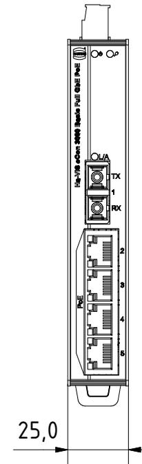
for mounting rail acc.to DIN EN 60715
