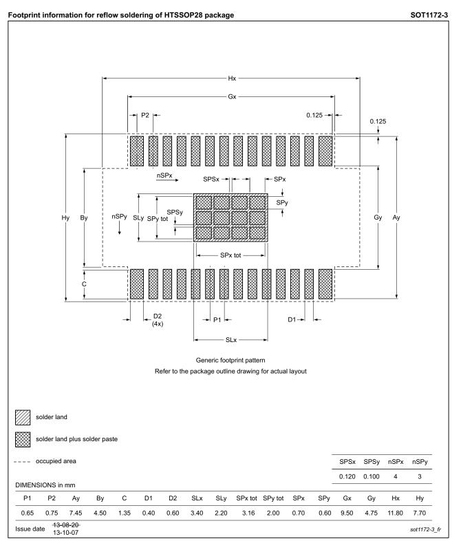
Fig 23. PCB footprint for SOT1172-3 (HTSSOP28); reflow soldering
