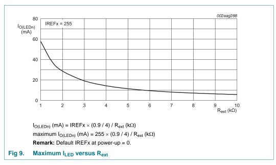
**Example 1:** If  $R_{ext}$  = 1  $k\Omega$ ,  $I_{O}$ \_LED\_MIN = 225  $\mu$ A,  $I_{O}$ \_LED\_MAX = 57.375 mA (as shown in Figure 10).
