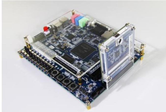
Figure 1-3 Connect the D8M to DE1-SoC board's expansion port
