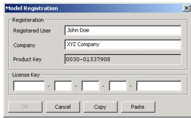
The Product Key is unique to each PC, and it is this information that is used to generate the License Key. Therefore, the Product Key must be provided at the time of order. To facilitate this process, you may click the Copy button, and then paste the information into the necessary forms during ordering.
