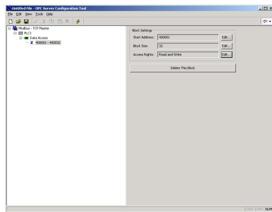
In the example above, we have configured the Start Address to **40001** to indicate that this is where we want the block to begin. We have also configured the Block Size to 32. Finally, we have configured the Access Rights as Read and Write, to indicate that we want the OPC client to be able to read and write data items exposed via this block.
