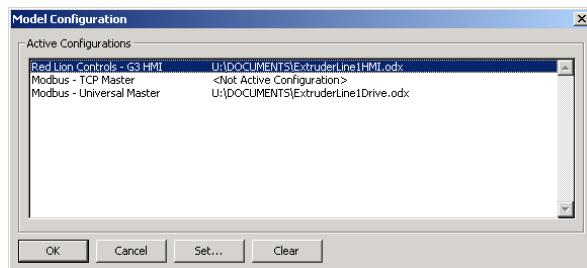
In the above example, the G3 – HMI and Modbus – Universal Master servers are configured, while the Modbus – TCP Master is not. To use a different configuration, click the Set button, and select a different file. If you want to disable an existing server, click the Clear button.
