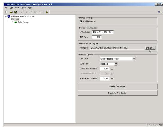
Finish by clicking the Data Access item on the left-hand pane, and then the Auto Configure button on the right-hand pane. The data items will be configured automatically, using the tag names from the cd2 file.
