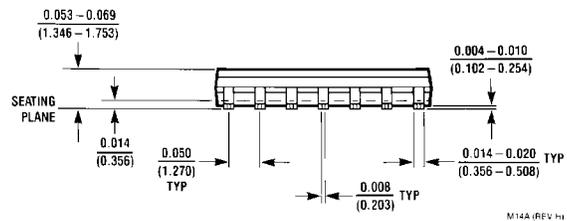
**14-Lead Small Outline Integrated Circuit (SOIC), JEDEC MS-012, 0.150" Narrow
