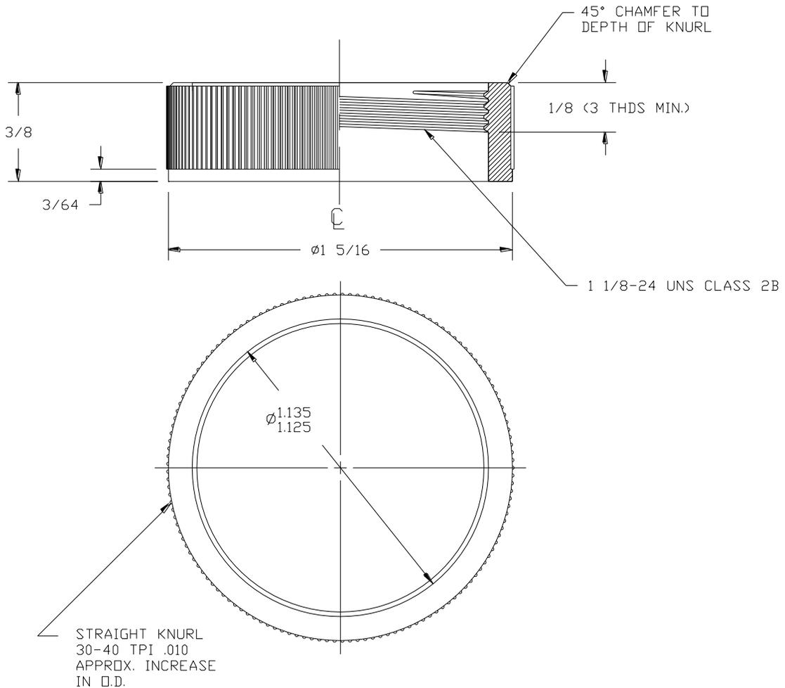
Start threads first or last depending on the panel thickness.
