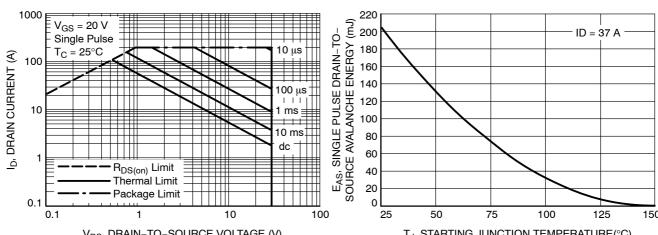
T<sub>J</sub>, STARTING JUNCTION TEMPERATURE(°C) V<sub>DS</sub>, DRAIN-TO-SOURCE VOLTAGE (V) Figure 11. Maximum Rated Forward Biased Figure 12. Maximum Avalanche Energy vs. Safe Operating Area **Starting Junction Temperature** (A) b V<sub>DS</sub> = 1.5 V 0.1 10,000 DRAIN CURRENT (A) PULSE WIDTH (µs) Figure 13. g<sub>FS</sub> vs. Drain Current Figure 14. I<sub>d</sub> vs. Pulse Width
