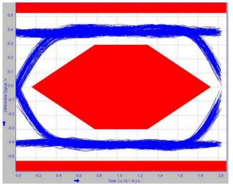
Figure 3. High Speed USB Eye Diagram of Signal Path without Switch
