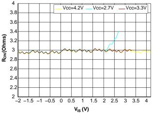
Figure 5. Audio ON Resistance vs. Signal Voltage @ T = 25°C, 2.7 V  $\leq$  V<sub>CC</sub>  $\leq$  4.2 V
