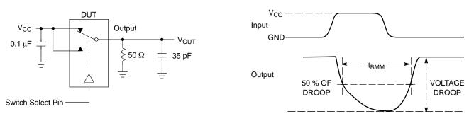
Figure 7. t<sub>BBM</sub> (Time Break-Before-Make)
