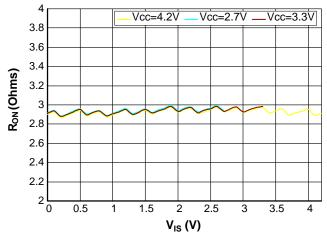
Figure 6. USB ON Resistance vs. Signal Voltage @ T = 25°C, 2.7 V  $\leq$  V<sub>CC</sub>  $\leq$  4.2 V
