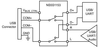
Figure 1. Application Diagram
