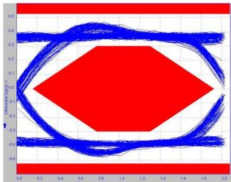
Figure 4. High Speed USB Eye Diagram of Signal Path with NS5S1153 (V<sub>CC</sub> = 3.6 V)
