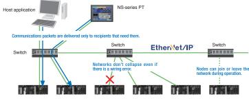
Star topology using Ethernet switch technology
