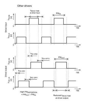
Figure 23(a). Timing Waveforms (Other Drivers)
