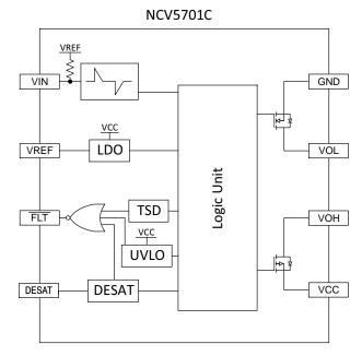
Figure 4(b). Simplified Block Diagram NCV5701C
