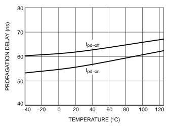
Figure 5. Propagation Delay vs. Temperature
