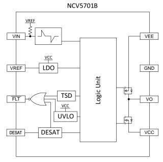
Figure 3(b). Simplified Block Diagram NCV5701B
