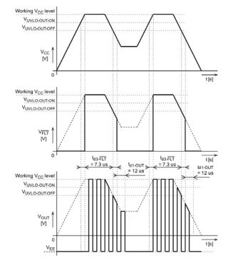
Figure 22. UVLO Function and Limits
