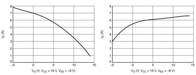
Figure 8. Output Source Current vs. Output Voltage
