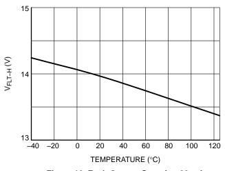
Figure 16. Fault Output, Sourcing 20 mA
