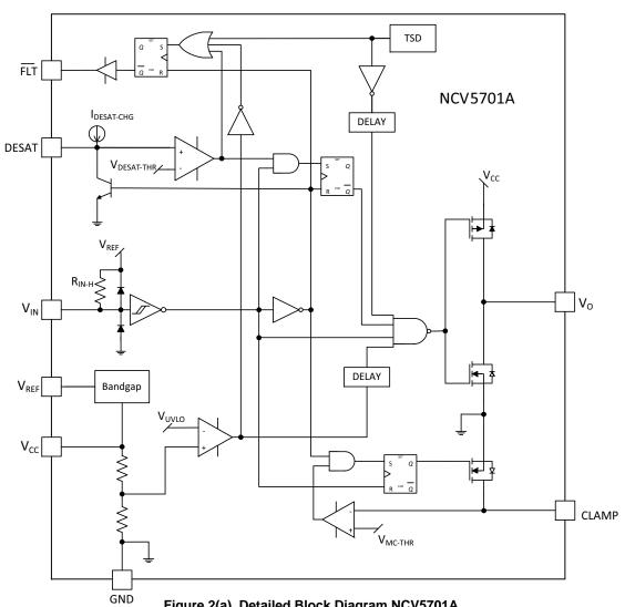
Figure 2(a). Detailed Block Diagram NCV5701A
