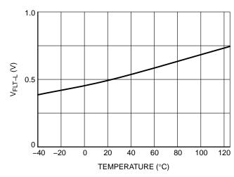
Figure 17. Fault Output, Sinking 15 mA
