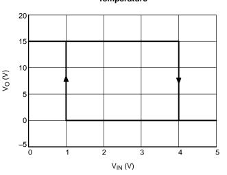
Figure 14. UVLO Threshold Voltages
