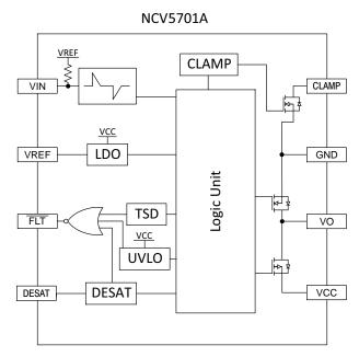
Figure 2(b). Simplified Block Diagram NCV5701A
