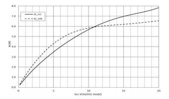
Figure 20. Output Current vs. Output Voltage Drop
