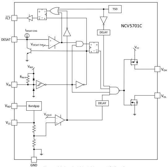
Figure 4(a). Detailed Block Diagram NCV5701C
