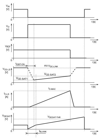
Figure 27. Desaturation Protection Waveforms
