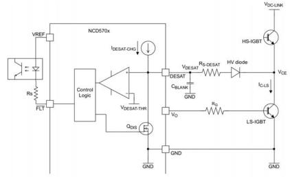
Figure 26. Desaturation Protection Schematic
