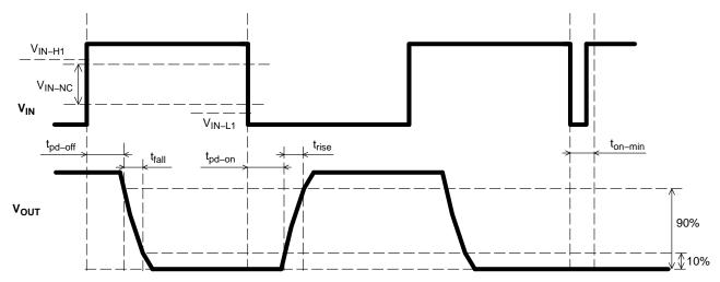
Figure 30. Input and Output Signal Parameters for Opto-coupler
