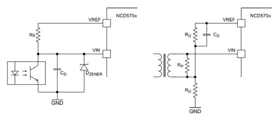
Figure 28. Opto-coupler or Pulse Transformer At Input
