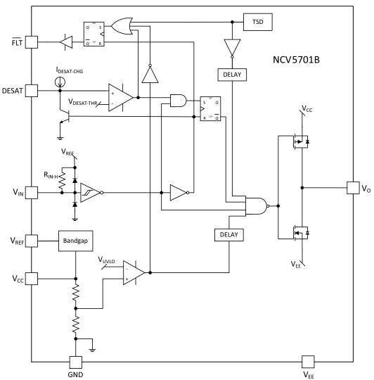
Figure 3(a). Detailed Block Diagram NCV5701B
