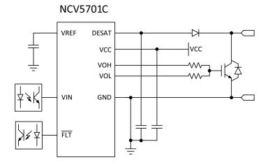
Figure 1. Simplified Application Schematics
