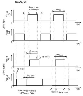
Figure 23(b). NCV5701 Timing Waveforms
