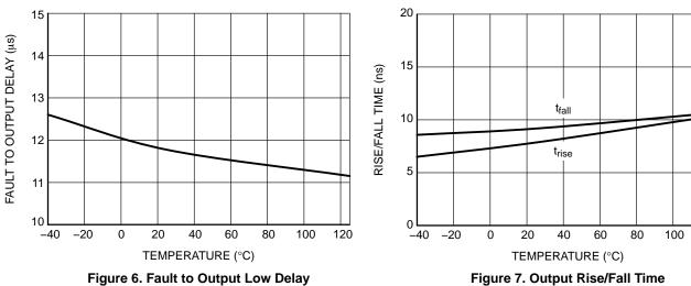
Figure 6. Fault to Output Low Delay
