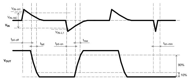
Figure 29. Input and Output Signal Parameters for Pulse Transformer
