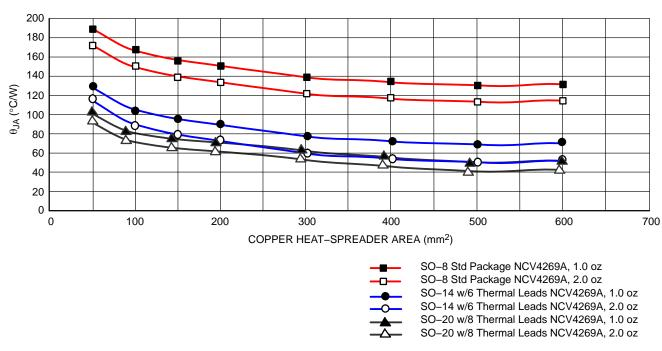
Figure 32. Junction–to–Ambient Thermal Resistance ( $\theta_{JA}$ ) vs. Heat Spreader Area
