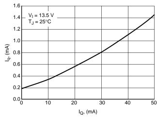
Figure 28. Current Consumption  $I_q$  vs. Output Current  $I_Q$
