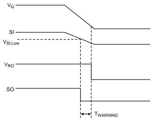
Figure 35. SO Warning Waveform Time Diagram
