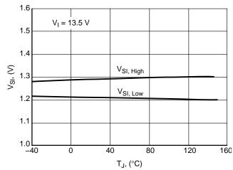
Figure 24. Sense Threshold  $V_{SI}$  vs. Temperature  $T_{J}$
