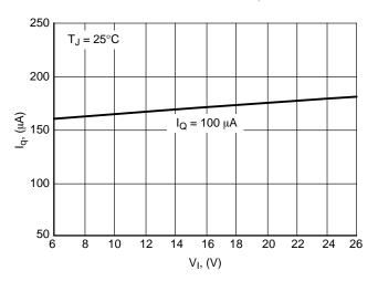
Figure 30. Quiescent Current  $I_q$  vs. Input Voltage  $V_I$
