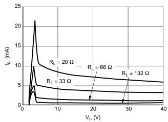
Figure 22. Current Consumption  $I_q$  vs. Input Voltage  $V_I$
