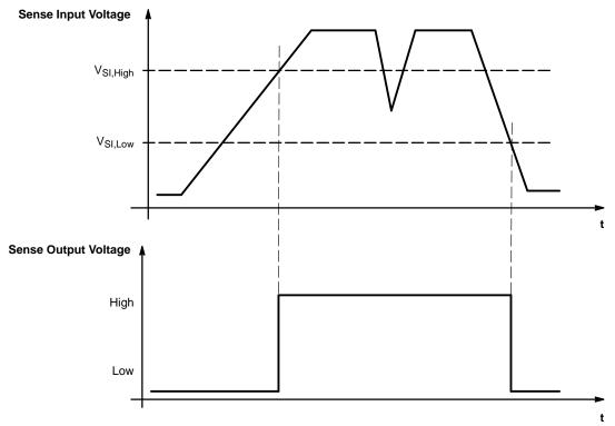
Figure 4. Sense Timing Diagram
