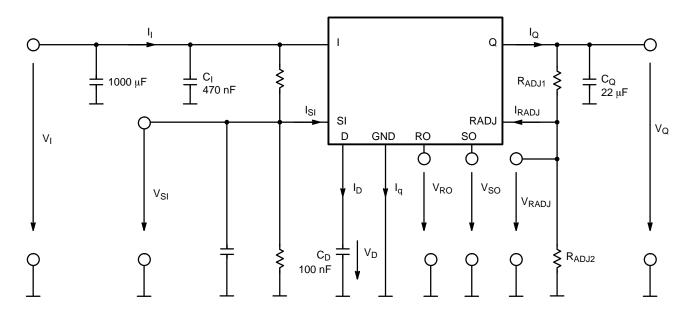
Figure 2. Measuring Circuit
