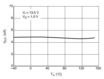
Figure 19. Charge Current I<sub>D.C</sub> vs. Temperature T<sub>J</sub>
