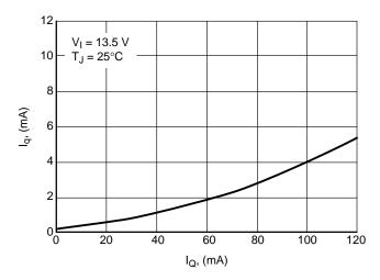
Figure 27. Current Consumption  $I_q$  vs. Output Current  $I_Q$
