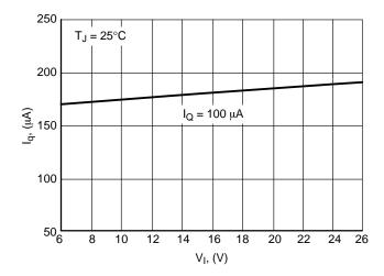
Figure 17. Quiescent Current  $I_q$  vs. Input Voltage  $V_I$
