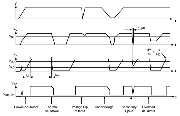
Figure 3. Reset Timing Diagram
