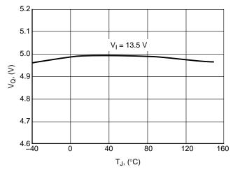
Figure 12. Output Voltage  $V_Q$  vs. Temperature  $T_J$
