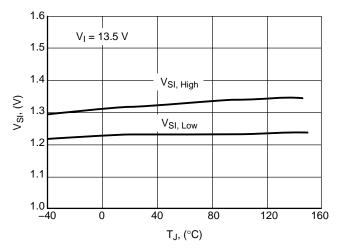
Figure 11. Sense Threshold  $V_{\text{SI}}$  vs. Temperature  $T_{\text{J}}$
