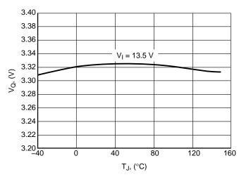
Figure 25. Output Voltage  $V_Q$  vs. Temperature  $T_J$
