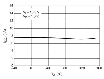
Figure 5. Charge Current  $I_{D,C}$  vs. Temperature  $T_J$
