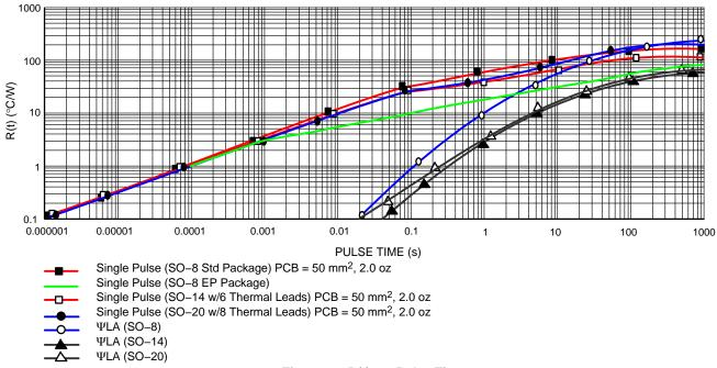
Figure 33. R(t) vs. Pulse Time
