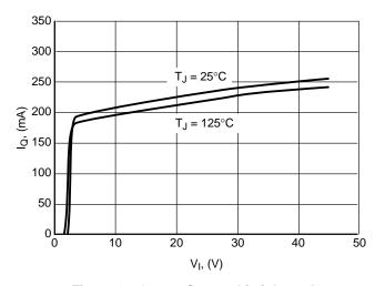
Figure 13. Output Current Limit  $I_Q$  vs. Input Voltage  $V_I$
