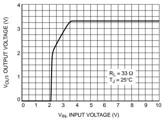
Figure 13. Output Voltage vs. Input Voltage (3.3 V Version)
