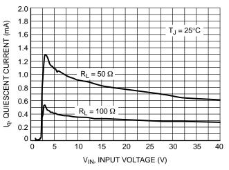
Figure 15. Quiescent Current vs. Input Voltage (3.3 V Version)
