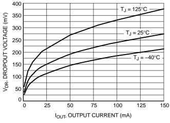
Figure 6. Dropout Voltage vs. Output Current (only 5.0 V Version)
