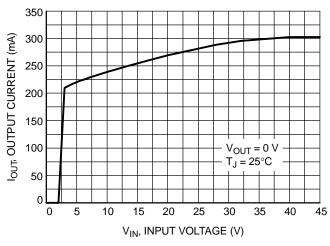
Figure 14. Maximum Output Current vs. Input Voltage (3.3 V Version)
