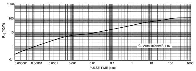
Figure 19. Single Pulse Heating Curve
