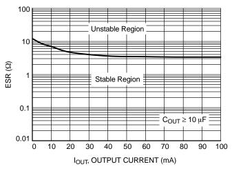
Figure 11. Output Stability with Output Capacitor ESR (3.3 V Version)
