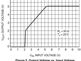
Figure 5. Output Voltage vs. Input Voltage (5.0 V Version)
