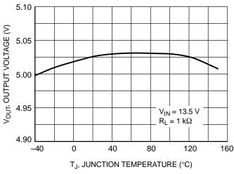
Figure 4. Output Voltage vs. Junction Temperature (5.0 V Version)
