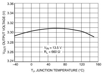
Figure 12. Output Voltage vs. Junction Temperature (3.3 V Version)
