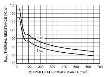
Figure 18.  $R_{\theta JA}$  vs. Copper Spreader Area
