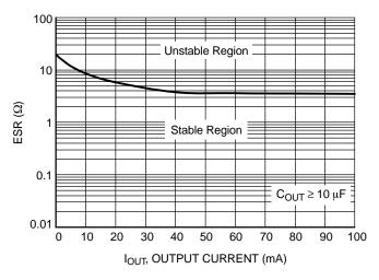
Figure 3. Output Stability with Output Capacitor ESR (5.0 V Version)
