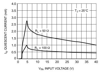
Figure 10. Quiescent Current vs. Input Voltage (5.0 V Version)
