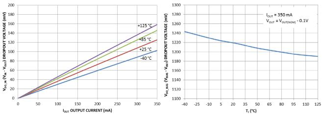
Figure 4. V<sub>IN</sub> Dropout Voltage vs. Output Current
