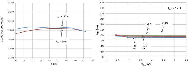
Figure 6. Output Voltage vs. Temperature
