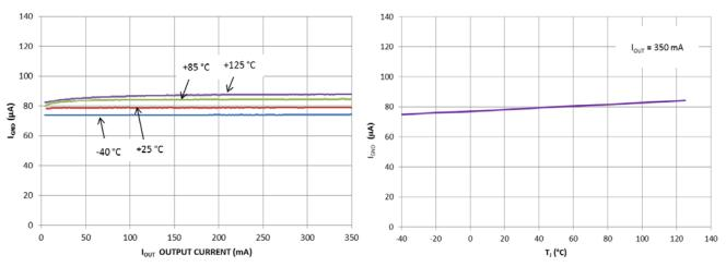
Figure 8. Bias Pin Current vs. Output Current
