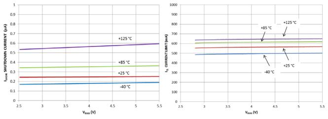
Figure 10. Shutdown Current vs. V<sub>BIAS</sub> Input Voltage
