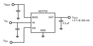
Figure 1. Typical Application Schematics
