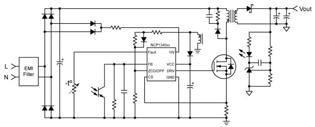
Figure 1. NCP1340 8-Pin Typical Application Circuit
