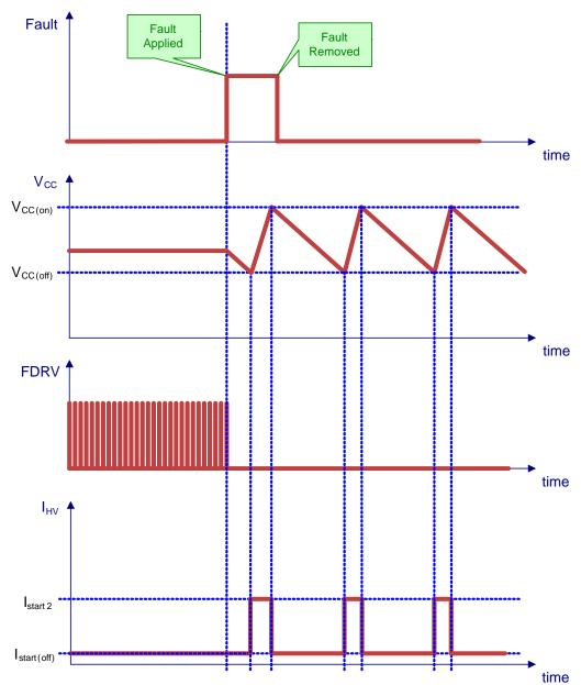
Figure 16. Operation During Latching Fault
