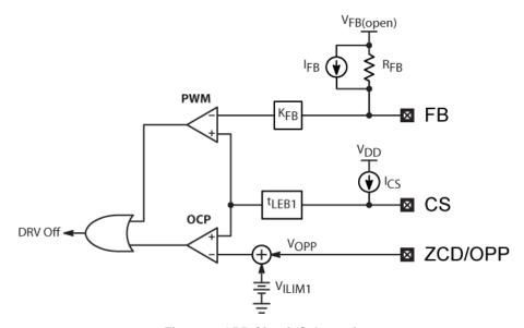
Figure 8. OPP Circuit Schematic
