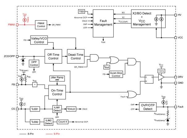
Figure 3. NCP1340 Block Diagram
