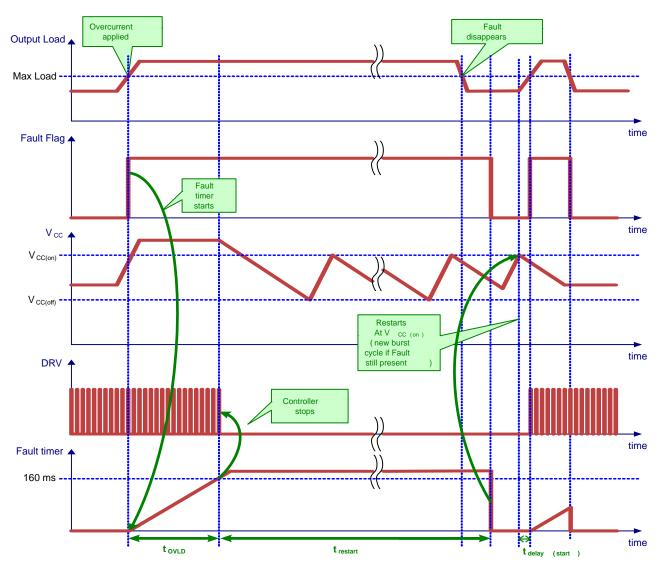
Figure 25. Auto-Recovery Overload Operation
