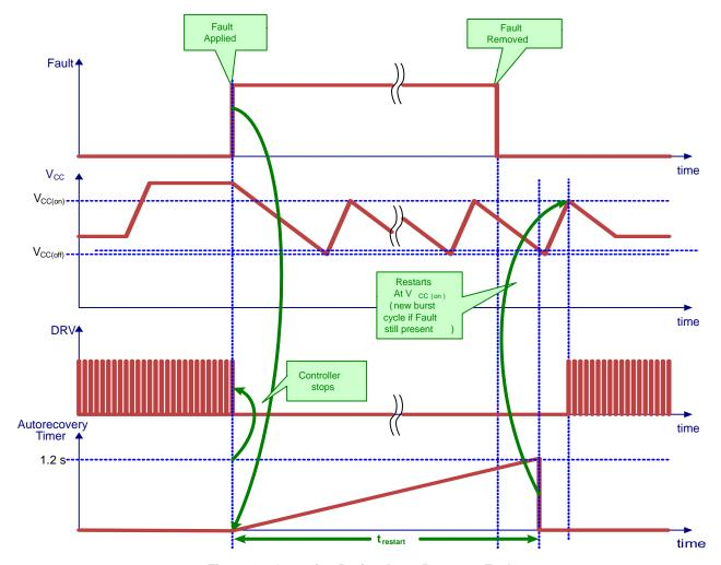
Figure 18. Operation During Auto-Recovery Fault
