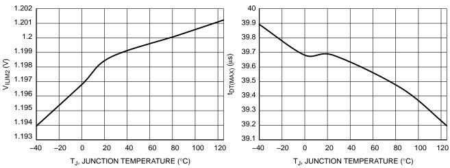
Figure 62.  $V_{ILIM2}$  vs. Temperature
