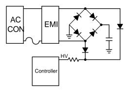
Figure 4. High-Voltage Input Connection
