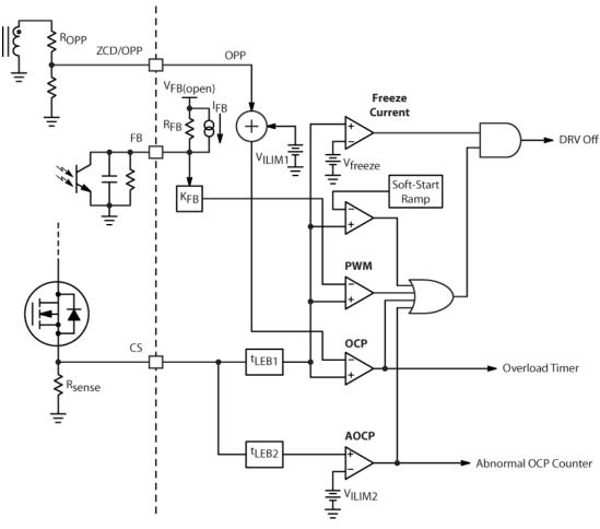
Figure 7. Current Sense Logic
