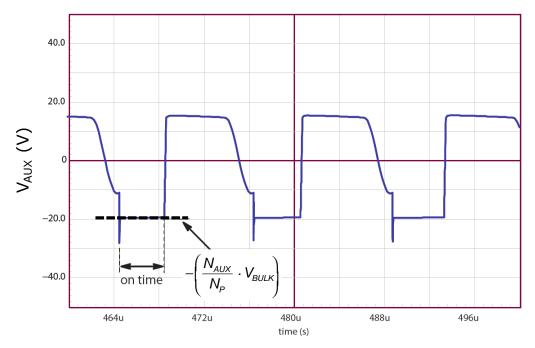
Figure 9. Auxiliary Winding Voltage
