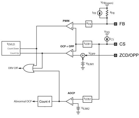
Figure 23. Overload Circuitry
