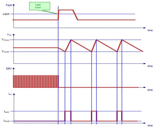
Figure 24. Latched Overload Operation
