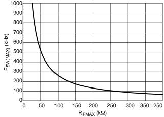
Figure 11. F<sub>SW(MAX)</sub> vs. R<sub>FMAX</sub>
