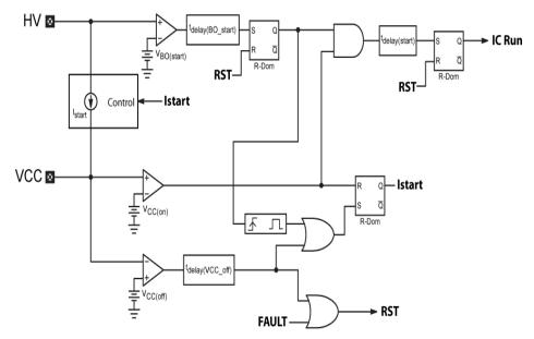
Figure 5. Start-up Circuitry Block Diagram
