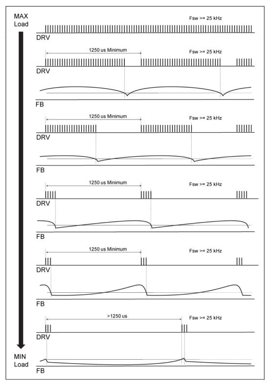
Figure 15. Quiet-Skip Timing Diagram
