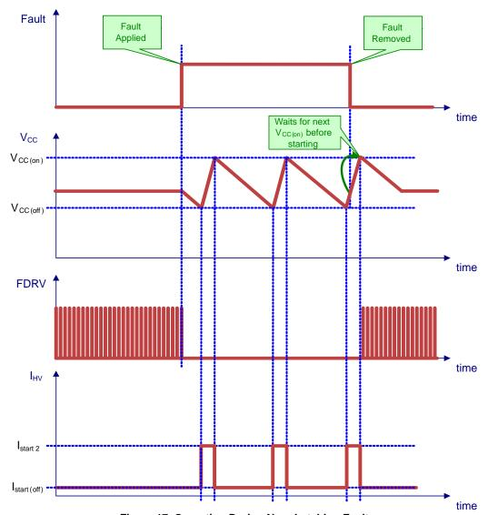
Figure 17. Operation During Non-Latching Fault
