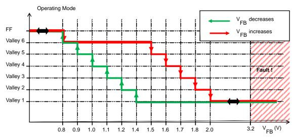
Figure 14. Valley Lockout Thresholds
