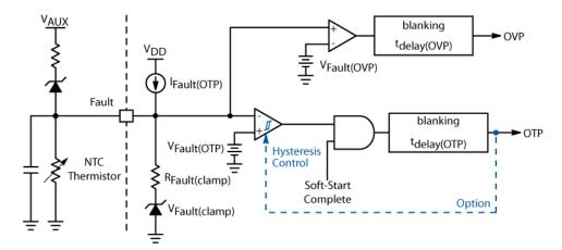
Figure 22. Fault Pin Internal Schematic
