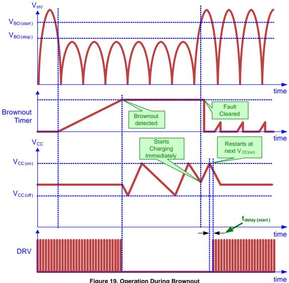
Figure 19. Operation During Brownout
