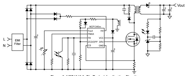
Figure 2. NCP1340 9-Pin Typical Application Circuit
