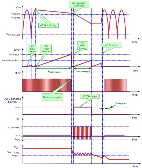
Figure 21. Line Removal Timing with AC Reapplied
