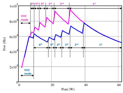
Figure 12. Valley Lockout Frequency vs. Output Power
