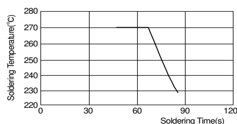
[Allowable Reflow Soldering Temperature and Time]
