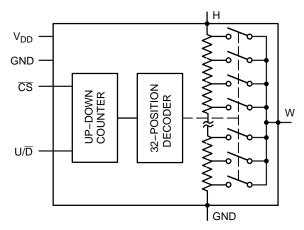
Figure 1. Functional Diagram
