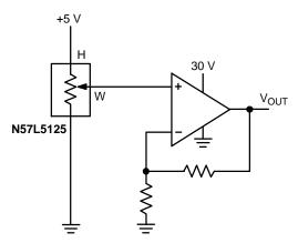
Figure 7. Positive LCD Bias Control
