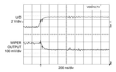
Figure 4. Tap-to-Tap Switching Transient
