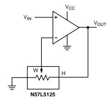
Figure 8. Adjustable Gain Circuit
