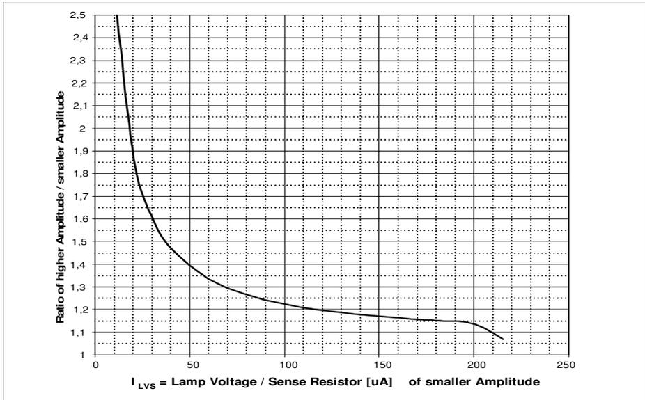
Figure 13 Maximum ratio of amplitudes versus sense current.
