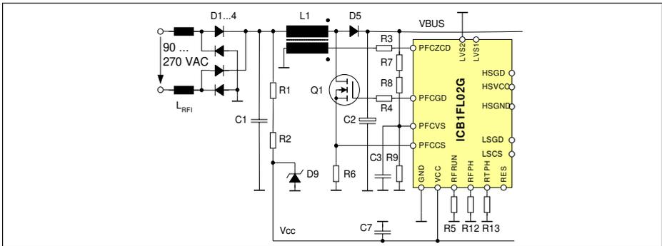
Figure 5 Circuit Diagram of the PFC preconverter section.
