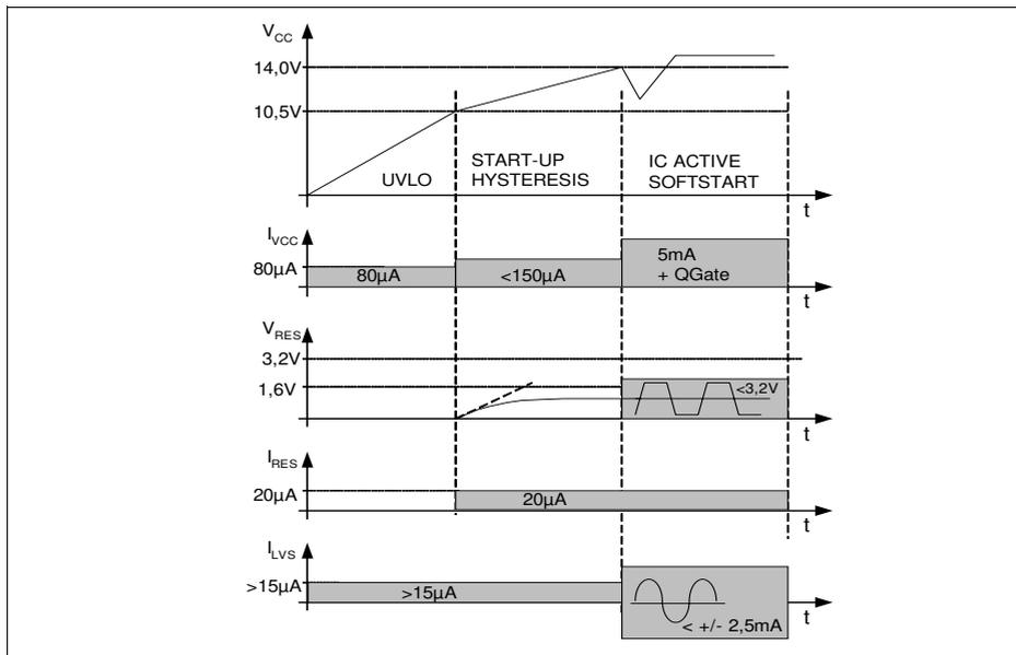
Figure 2 Progress of levels during a typical start-up.
