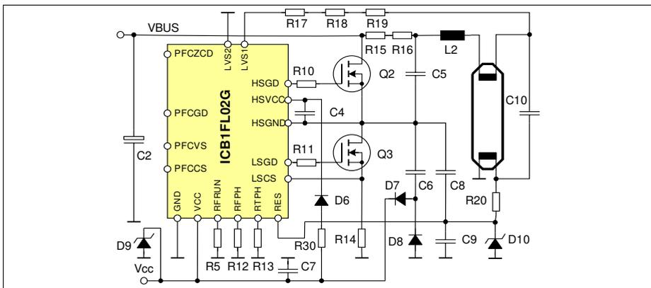
Figure 11 Circuit diagram of the lamp inverter section.
