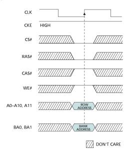
Figure 8: Meeting <sup>t</sup>RCD (MIN) When 2 < <sup>t</sup>RCD (MIN)/<sup>t</sup>CK< 3
