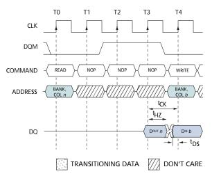
Notes: 1. CL = 3 is used for illustration; the READ command may be to any bank, and the WRITE command may be to any bank. If a burst of one is used, then DQM is not required.
