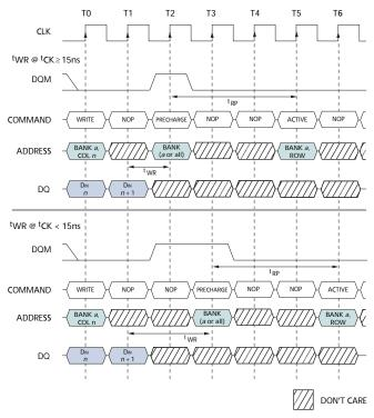
Notes: 1. DQM could remain LOW in this example if the WRITE burst is a fixed length of two.
