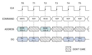
Notes: 1. CL = 2 is used for illustration; the WRITE command may be to any bank, and the READ command may be to any bank. DQM is LOW.
