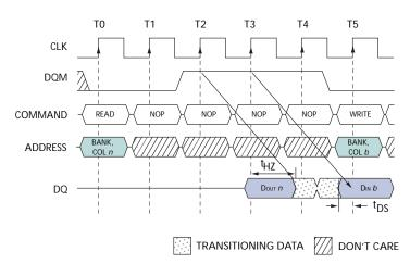
Notes: 1. CL = 3 is used for illustration; the READ command may be to any bank, and the WRITE command may be to any bank.
