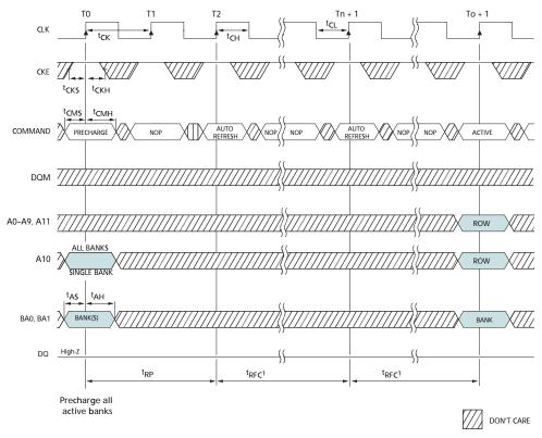
Notes: 1. Each AUTO REFRESH command performs a REFRESH cycle. Back-to-back commands are not required. <sup>t</sup>RFC must not be interrupted by any executable command; COMMAND INHIBIT or NOP must be applied on each positive edge during <sup>t</sup>RFC.
