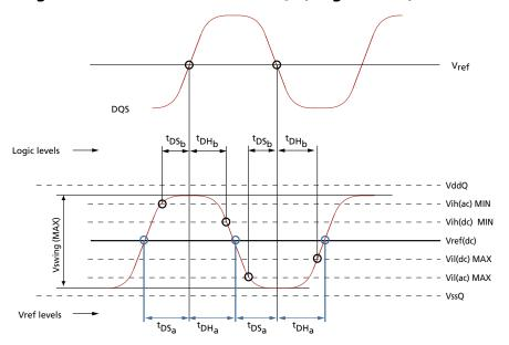
Figure 37: AC Input Test Signal Waveform (Differential)
