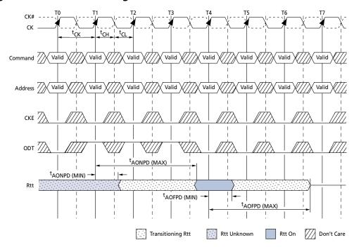
Figure 87: ODT Turn-Off Timings When Entering Power-Down Mode
