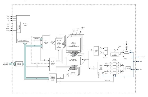
Figure 5: 64 Meg x 16 Functional Block Diagram
