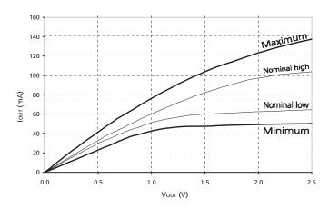
Figure 12: Full Drive Pull-Up Characteristics
