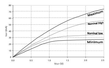
Figure 14: Reduced Drive Pull-Up Characteristics
