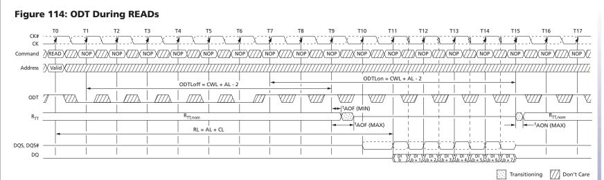
Note: 1. ODT must be disabled externally during READs by driving ODT LOW. For example, CL = 6; AL = CL - 1 = 5; RL = AL + CL = 11; CWL = 5; ODTLon = CWL + AL - 2 = 8; ODTLoff = CWL + AL - 2 = 8. R<sub>TT,nom</sub> is enabled. R<sub>TT(WR)</sub> is a "Don't Care."
