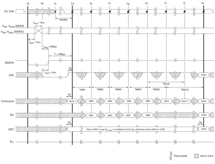
Note: 1. From time point Td until Tk, NOP or DES commands must be applied between MRS and ZQCL commands.
