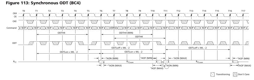
Notes: 1. WL = 7.  $R_{TT,nom}$  is enabled.  $R_{TT(WR)}$  is disabled.
