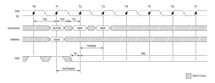
Figure 103: PRECHARGE to Power-Down Entry
