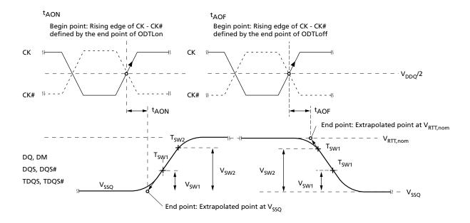
Figure 24: <sup>t</sup>AONPD and <sup>t</sup>AOFPD Definitions
