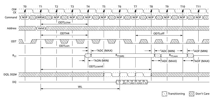
Notes: 1. Via MRS or OTF. AL = 0, CWL = 5.  $R_{TT,nom}$  and  $R_{TT(WR)}$  are enabled.
