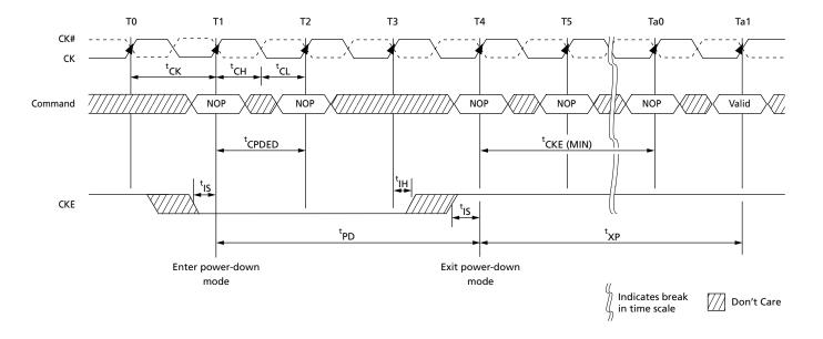
Figure 97: Precharge Power-Down (Slow-Exit Mode) Entry and Exit
