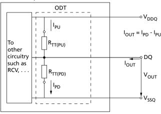
**Table 32: On-Die Termination DC Electrical Characteristics**
