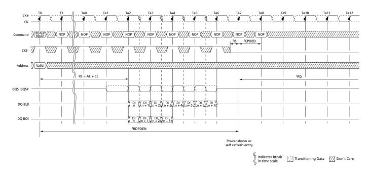
Figure 99: Power-Down Entry After WRITE
