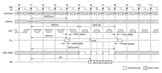
Notes: 1. Via MRS or OTF. AL = 0, CWL = 5.  $R_{TT,nom}$  can be either enabled or disabled. If disabled, ODT can remain HIGH.  $R_{TT(WR)}$  is enabled.
