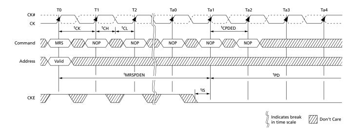
Figure 105: Power-Down Exit to Refresh to Power-Down Entry
