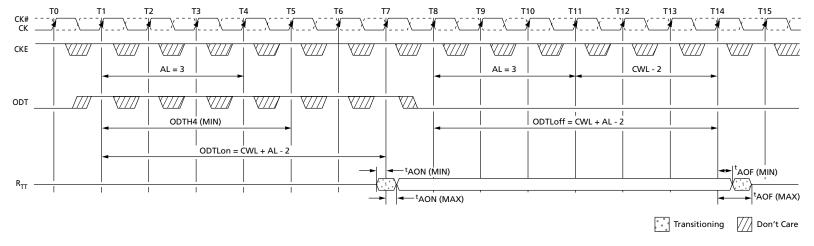
Note: 1. AL = 3; CWL = 5; ODTLon = WL = 6.0; ODTLoff = WL - 2 = 6.  $R_{TT,nom}$  is enabled.
