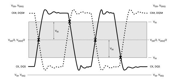
Figure 17: Single-Ended Requirements for Differential Signals
