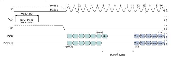
Note: 1. Xb is the XIP confirmation bit and should be set as follows: 0 to keep XIP state; 1 to exit XIP mode and return to standard read mode.
