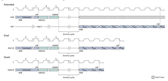
Note: 1. For extended SPI protocol,  $C_x = 7 + (A[MAX] + 1)$ ; For dual SPI protocol,  $C_x = 3 + (A[MAX] + 1)/2$ ; For quad SPI protocol,  $C_x = 1 + (A[MAX] + 1)/4$ .
