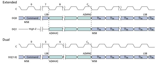
Notes: 1. For extended SPI protocol,  $C_x = 7 + (A[MAX] + 1)/2$ ; For dual SPI protocol,  $C_x = 3 + (A[MAX] + 1)/2$ .
