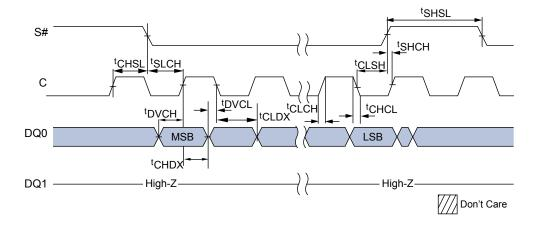
Figure 45: Write Protect Setup and Hold During WRITE STATUS REGISTER Operation (SRWD = 1)
