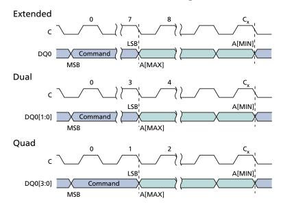
Notes: 1. For extended SPI protocol,  $C_x = 7 + (A[MAX] + 1)$ ; For dual SPI protocol,  $C_x = 3 + (A[MAX] + 1)/2$ ; For quad SPI protocol,  $C_x = 1 + (A[MAX] + 1)/4$ .
