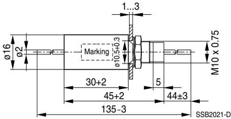
Tightening torque: 3 +0.5 Nm
