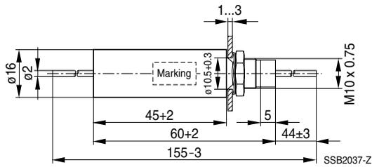
Tightening torque: 3 +0.5 Nm
