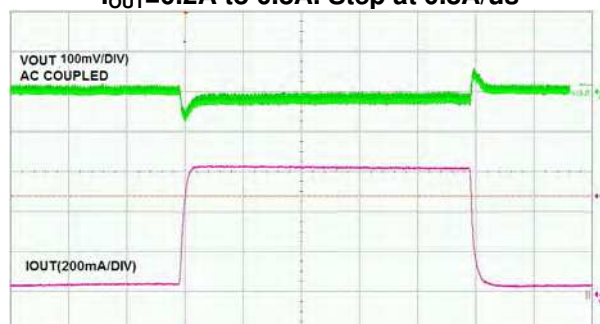
Load Transient Test I_{OUT}=0.2A to 0.8A . Step at 0.8A/\mu s
