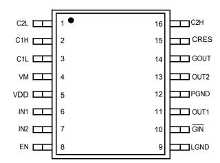
Figure 3. VMFP Pin Connections
