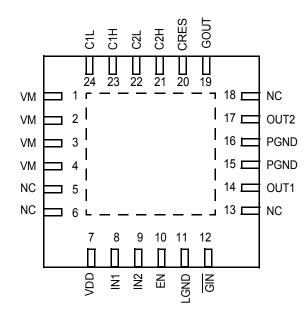
Figure 4. QFN Pin Connections
