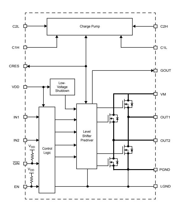
Figure 2. 17511A Simplified Internal Block Diagram
