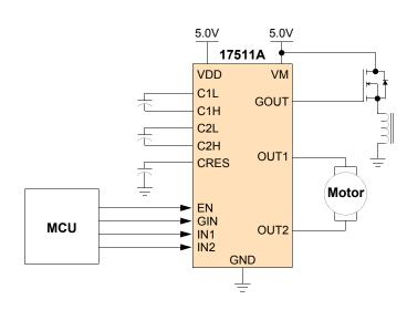
Figure 1. 17511A Simplified Application Diagram
