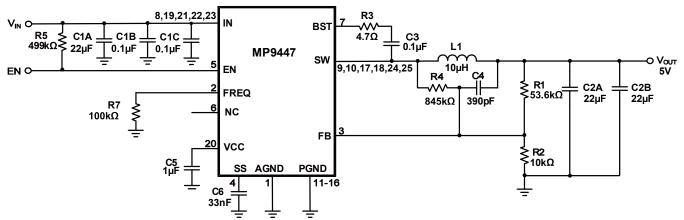
Figure 11: Typical Application Circuit, 5V-Output
