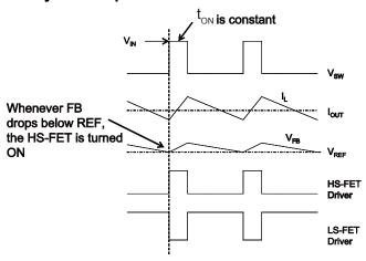
Figure 2: Heavy-Load Operation
