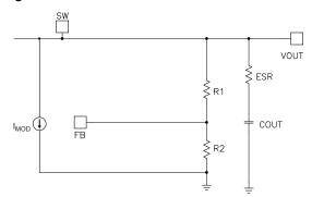
Figure 8: Simplified Circuit in Skip Mode
