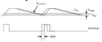
Figure 5: Jitter in Skip Mode
