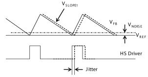
Figure 4: Jitter in PWM Mode
