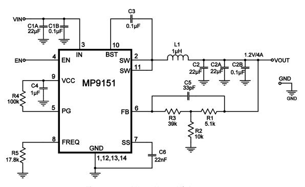
Figure 11: 800kHz, 12V<sub>IN</sub>, 1.2V/4A Output
