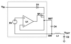
Figure 4: Internal Bootstrap Charging Circuit
