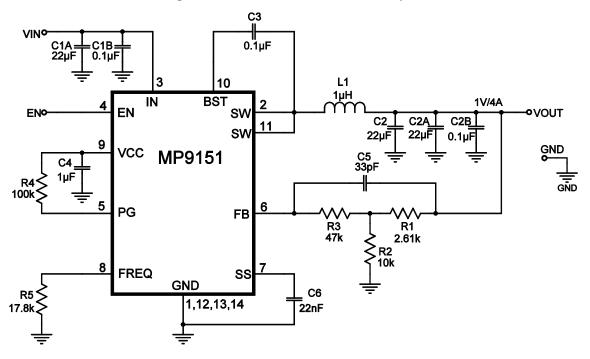
Figure 12: 800kHz, 12V<sub>IN</sub>, 1V/4A Output
