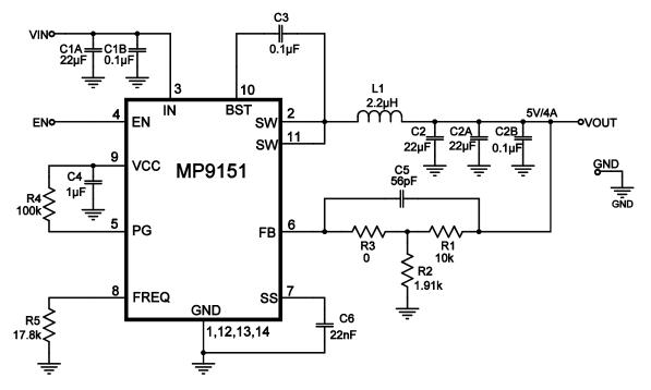
Figure 7: 800kHz, 12V<sub>IN</sub>, 5V/4A Output
