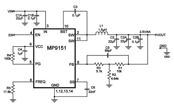
Figure 9: 800kHz, 12V<sub>IN</sub>, 2.5V/4A Output
