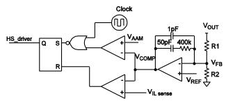
Figure 3: Simplified AAM Control Logic
