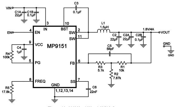
Figure 10: 800kHz, 12V<sub>IN</sub>, 1.8V/4A Output
