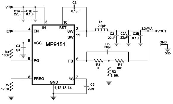
Figure 8: 800kHz, 12V<sub>IN</sub>, 3.3V/4A Output
