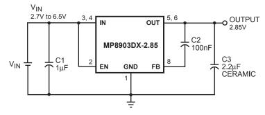
Figure 3—Typical Application Circuit (Fixed)
