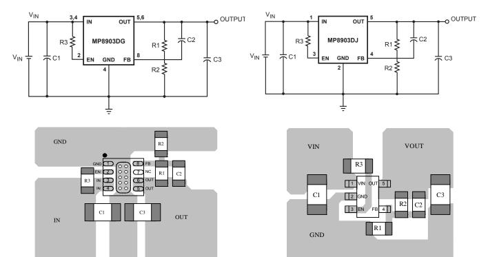
Top Layer Figure 5—PCB Layout
