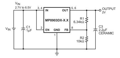
Figure 4—Typical Application Circuit (Adjustable)
