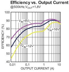
Figure 40 — Efficiency Curve
