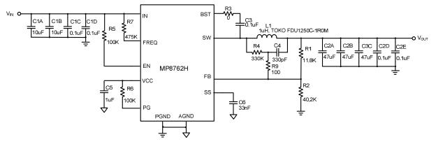
Figure 21 — Typical Application Circuit with Low ESR Ceramic Capacitor  $V_{IN}$ =12V,  $V_{OUT}$ =0.8V,  $I_{OUT}$ =10A,  $F_{SW}$ =300kHz
