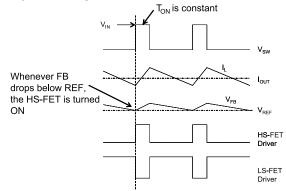
Figure 2—Heavy Load Operation
