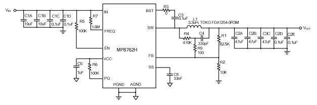
Figure 51 — Typical Application Circuit with Low ESR Ceramic Capacitor  $V_{IN}$ =12V,  $V_{OUT}$ =5 V,  $I_{OUT}$ =10A,  $F_{SW}$ =500kHz
