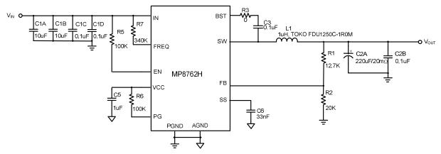
Figure 13 — Typical Application Circuit with No External Ramp
