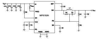
Figure 55—Schematic for PCB Layout Guide
