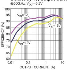
Figure 46 — Efficiency Curve
