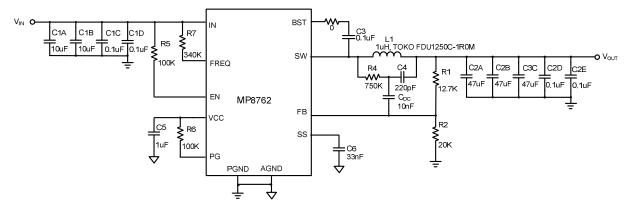
Figure 15 — Typical Application Circuit with Low ESR Ceramic Capacitor and DC-Blocking Capacitor.
