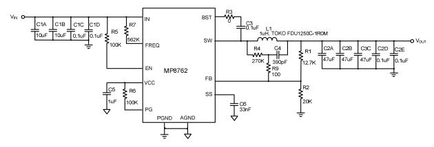
Figure 17 — Typical Application Circuit with Low ESR Ceramic Capacitor
