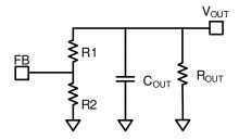
Figure 8—Simplified Circuit in skip Mode
