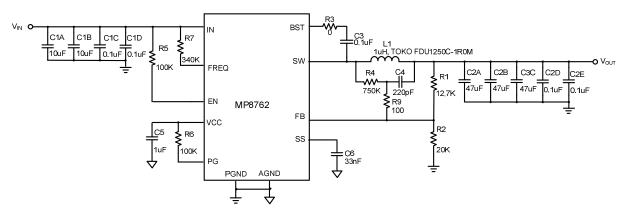
Figure 14 — Typical Application Circuit with Low ESR Ceramic Capacitor  $V_{\text{IN}}$ =12V,  $V_{\text{OUT}}$ =1V,  $I_{\text{OUT}}$ =10A,  $F_{\text{SW}}$ =500kHz
