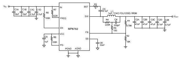
Figure 27 — Typical Application Circuit with Low ESR Ceramic Capacitor  $V_{IN}=12V,\ V_{OUT}=1.2V,\ I_{OUT}=10A,\ F_{SW}=500kHz$
