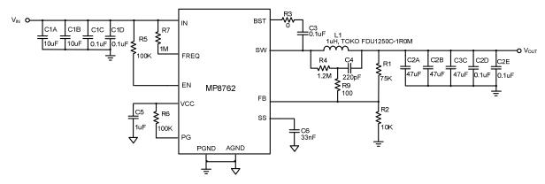
Figure 53 — Typical Application Circuit with Low ESR Ceramic Capacitor  $V_{IN}$ =12V,  $V_{OUT}$ =5 V,  $I_{OUT}$ =10A,  $F_{SW}$ =800kHz
