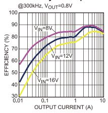
Figure 22 — Efficiency Curve
