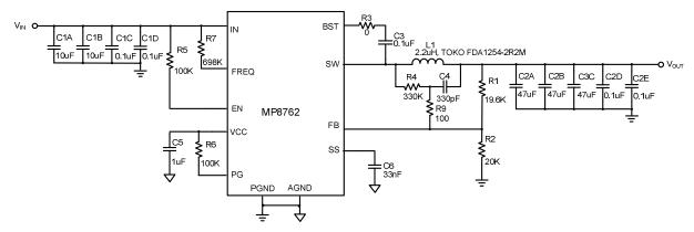
Figure 25 — Typical Application Circuit with Low ESR Ceramic Capacitor
