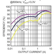
Figure 48 — Efficiency Curve
