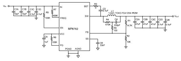
Figure 33 — Typical Application Circuit with Low ESR Ceramic Capacitor  $V_{IN}=12V,\ V_{OUT}=1.5\ V,\ I_{OUT}=10A,\ F_{SW}=500kHz$
