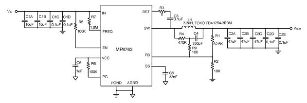
Figure 51 — Typical Application Circuit with Low ESR Ceramic Capacitor  $V_{\text{IN}}$ =12V,  $V_{\text{OUT}}$ =5 V,  $I_{\text{OUT}}$ =10A,  $F_{\text{SW}}$ =500kHz
