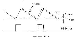
Figure 4—Jitter in PWM Mode
