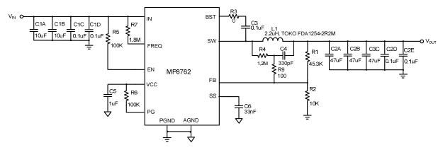
Figure 43 — Typical Application Circuit with Low ESR Ceramic Capacitor
