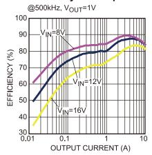
Figure 16 — Efficiency Curve
