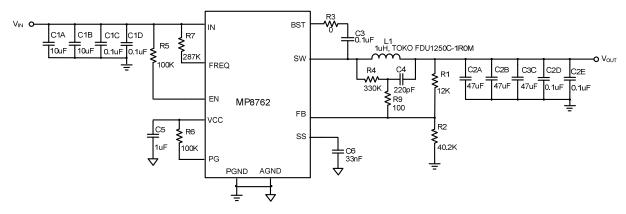
Figure 23 — Typical Application Circuit with Low ESR Ceramic Capacitor
