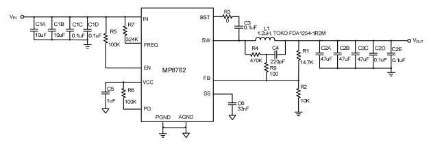
Figure 35 — Typical Application Circuit with Low ESR Ceramic Capacitor
