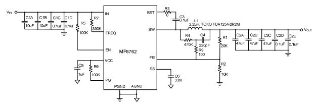
Figure 41 — Typical Application Circuit with Low ESR Ceramic Capacitor
