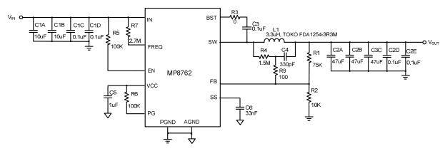
Figure 49 — Typical Application Circuit with Low ESR Ceramic Capacitor
