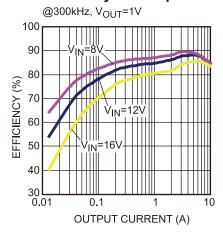
Figure 18 — Efficiency Curve
