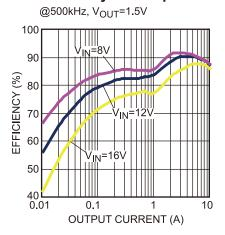
Figure 34 — Efficiency Curve
