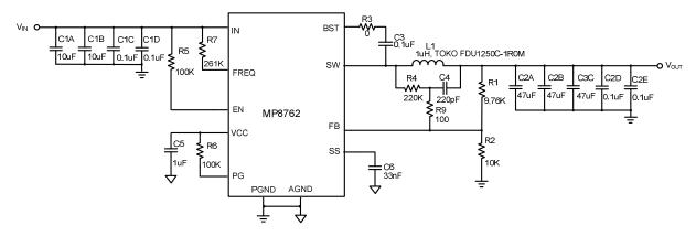
Figure 29 — Typical Application Circuit with Low ESR Ceramic Capacitor
