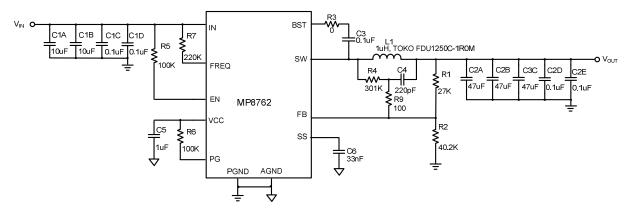
Figure 19 — Typical Application Circuit with Low ESR Ceramic Capacitor
