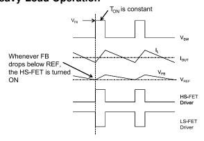
Figure 2—Heavy Load Operation
