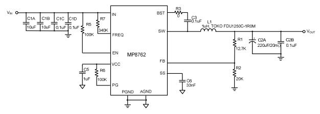
Figure 13 — Typical Application Circuit with No External Ramp  $V_{\text{IN}}$ =12V,  $V_{\text{OUT}}$ =1V,  $I_{\text{OUT}}$ =10A,  $F_{\text{SW}}$ =500kHz
