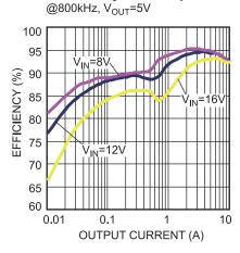
Figure 54 — Efficiency Curve  $V_{\text{OUT}}$ =5V,  $I_{\text{OUT}}$ =0.01A-10A,  $F_{\text{SW}}$ =800kHz
