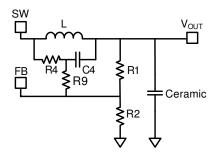
Figure11—Simplified Circuit of Ceramic Capacitor
