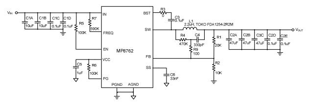
Figure 39 — Typical Application Circuit with Low ESR Ceramic Capacitor  $V_{IN}=12V, V_{OUT}=1.8 V, I_{OUT}=10A, F_{SW}=500kHz$
