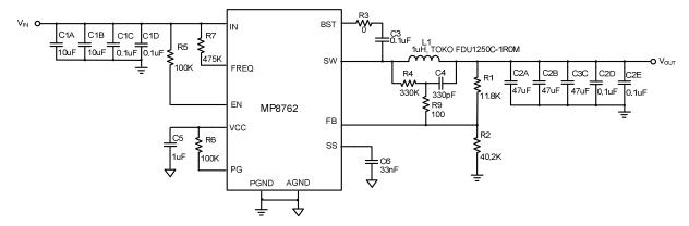
Figure 21 — Typical Application Circuit with Low ESR Ceramic Capacitor  $V_{\text{IN}}$ =12V,  $V_{\text{OUT}}$ =0.8V,  $I_{\text{OUT}}$ =10A,  $F_{\text{SW}}$ =300kHz
