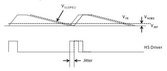
Figure 5—Jitter in Skip Mode
