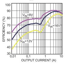
Figure 42 — Efficiency Curve
