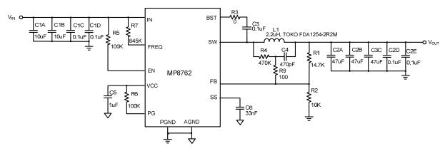
Figure 31 — Typical Application Circuit with Low ESR Ceramic Capacitor
