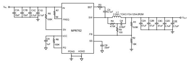
Figure 37 — Typical Application Circuit with Low ESR Ceramic Capacitor
