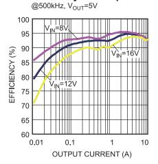
Figure 52 — Efficiency Curve V<sub>OUT</sub>=5V, I<sub>OUT</sub>=0.01A-10A, F<sub>SW</sub>=500kHz
