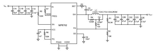
Figure 45 — Typical Application Circuit with Low ESR Ceramic Capacitor  $V_{\text{IN}}$ =12V,  $V_{\text{OUT}}$ =3.3 V,  $I_{\text{OUT}}$ =10A,  $F_{\text{SW}}$ =500kHz
