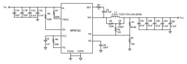
Figure 47 — Typical Application Circuit with Low ESR Ceramic Capacitor
