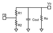
Figure 8—Simplified Circuit in skip Mode
