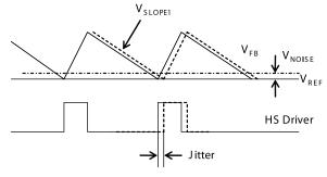
Figure 4—Jitter in PWM Mode
