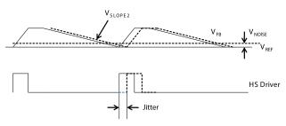
Figure 5—Jitter in Skip Mode
