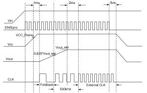
Figure 4—Startup Sequence Using External Sync Clock Signal
