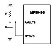
Figure 1—Fault Protection Enhancement Circuit
