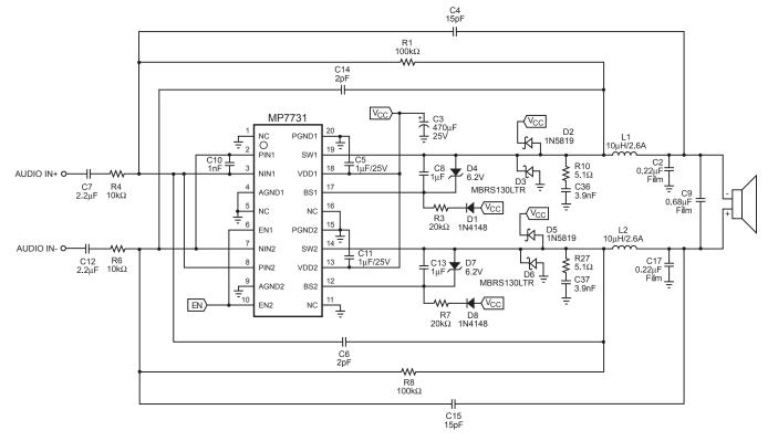
Figure 1— Mono Full Bridged Circuit
